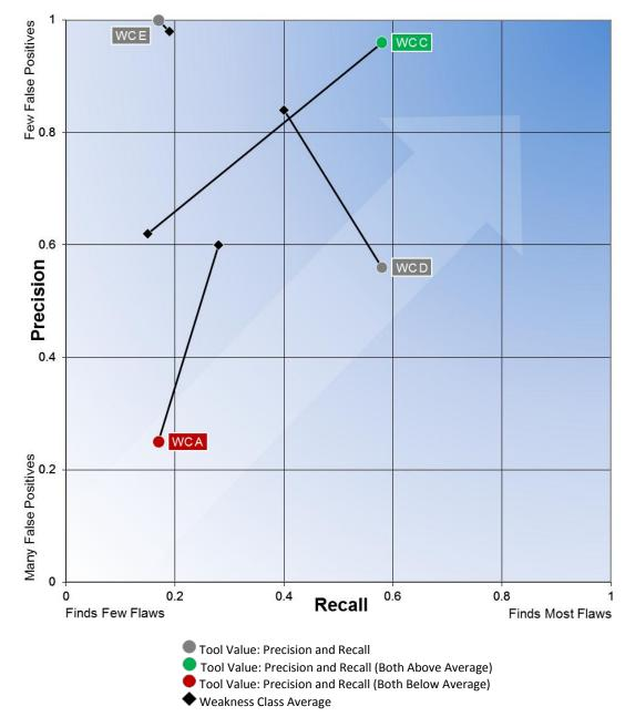
Figure 3 – Example Precision-Recall Graph for single tool
