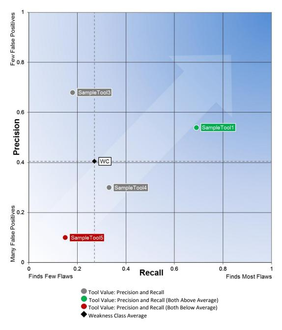
Figure 7 – Example Precision-Recall Graph for Weakness Class (WC)
